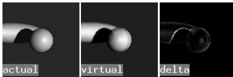
FIGURE 12.7. Virtual view within the span. A virtual view positioned midway between the center and left basis images is well within the span of the basis set. In this figure (and the series of figures that follow) both the rendering of the desired view (left) and the view interpolated from the basis set (center) are presented. On the right is the absolute value of difference between the two images scaled to the range 0 to 255. The combined errors from rendering, warping and defocus are generally small and are largest at interposition boundaries. Problems are concentrated at depth discontinuities because of aliasing in the rendering, relatively large changes in the surface sampling of steep gradients as seen from the virtual view, and the spread of blur circles across object boundaries even though the surfaces lie at different depths.
