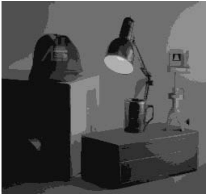
Figure 7: Contribution of Different Sensitivities to Composite Image. Reflecting the large range of intensities, the composite image is a mosaic of regions of varying quantization resolution. The grey scale in this image is proportional to the size of the quantization interval in the respective source images. In those portions of the image with higher luminance, sensitivity is decreased in order to extend the range of representation. In the darker portions of the image, the decreased range requirements allow greater resolution.
